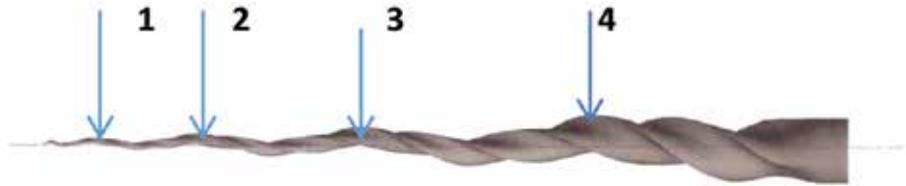
Figure 13: Localized compression testing was performed at four points along the length of the X-File as shown
