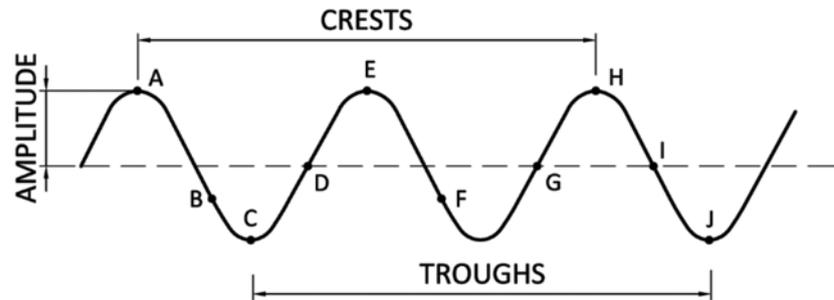
Figure 1: Depicts a transverse wave, which consists of oscillations occurring perpendicular or at right angles to the direction of the wave. The waves are composed of crests and troughs with a specific amplitude that determines the energy or force transmitted by each wave
