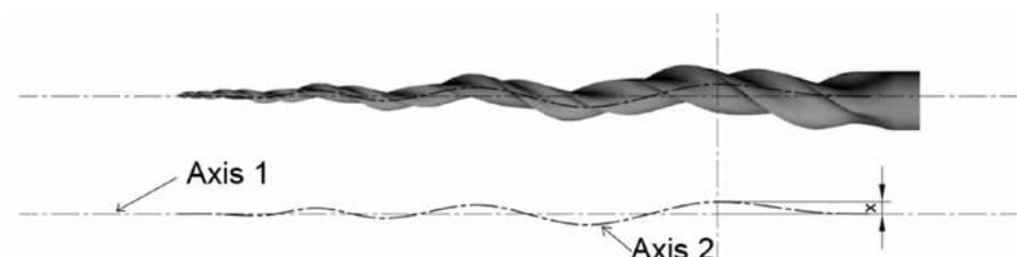
Figure 5: A schematic of the profile and dual axis of Protaper NEXT. Axis 1 is the central or rotational axis, and Axis 2 is the cutting or precessional axis. The distance-X between the two axes decrease continuously from shank to tip, where the axes meet, leaving the tip completely centered. The offset center of mass, inherent in this design, enables the X-File to cut precessionally
