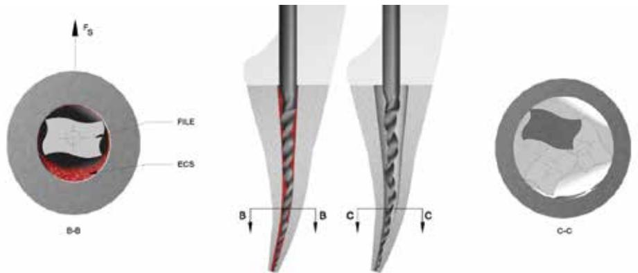
Figures 8-9: Demonstrates the instrument in its constrained or compressed condition. When the file is fully constrained,  $x$  (as shown in Figure 5), which represents the deflection of the file due to  $F$ , would initially be zero or nearly zero. Demonstrates the file's tendency will be to return to the natural or uncompressed state in which it is precessing about its central axis
