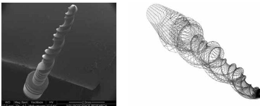
Figures 3-4: An SEM of the profile and an Auto-CAD image of the X-File demonstrating the spring or coil-like profile of the instrument
