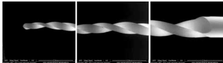
Figures 10A -10C: Scanning electron micrograph of the instrument itself demonstrating the nodes of the file and the instrument in the unconstrained or uncompressed condition
