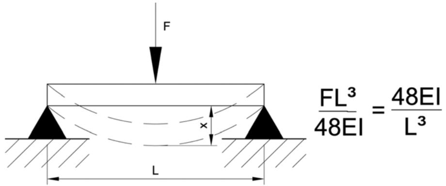
Figure 7: A schematic of a simply supported beam and the equation used to determine the stiffness or restoring force of the simply supported beam (where  $x$  is the maximum deflection)
