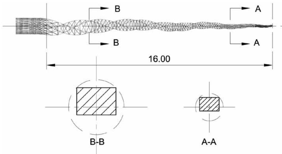
Figure 2: A schematic of offset rectilinear cross section of ProTaper NEXT. As can be seen from this figure, only two cutting angles engage the walls of the root canal at any one time. This offset rectilinear cross section not only contributes to the innate flexibility of the file, but also permits intermittent cutting, which mitigates cyclic fatigue. The large clearance angle opposite the cutting flutes facilitates hauling and elimination of debris
