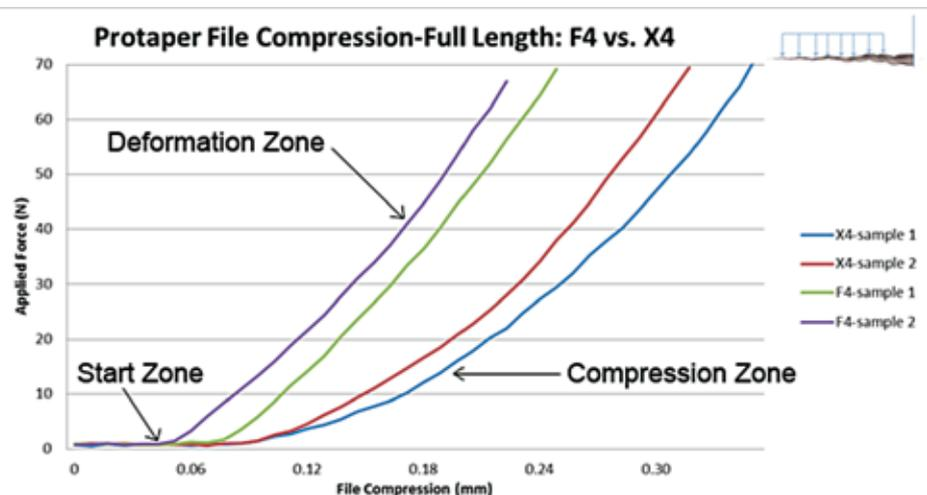
Figure 12: Shows a data plot comparison from the compression testing of the X4-File versus the F4-File. This plot is representative of the data plots of all of the files sizes tested. The response of the X-File to the applied load is clearly different from that of the F-File. For analysis purposes, the plot is divided into three zones as labeled in Figure 12
